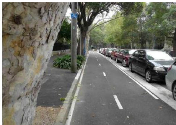
Figure 8: Bidirectional bicycle path protected by car parking in Sydney 26
